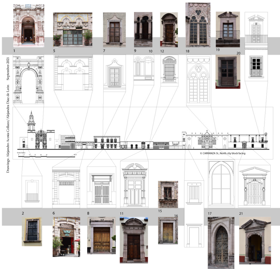
Figure 2: Typology of Carranza St. openings (windows and entrances, north city block facing). (Source: Author's research, 2021. Drawing made and edited by Alejandro Acosta Collazo and Alejandra Díaz de León Esparza. Photographs by Jéssica González Reyes, September 14th 2021.)
